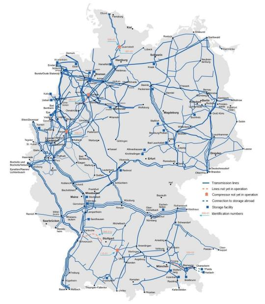
Figure 106 Gas transmission grid Germany (overview)
