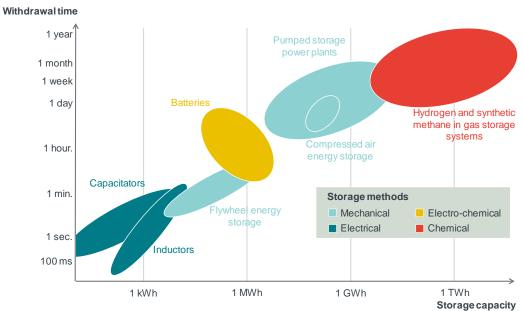
Figure 24 Schematic comparison of energy storage technologies
