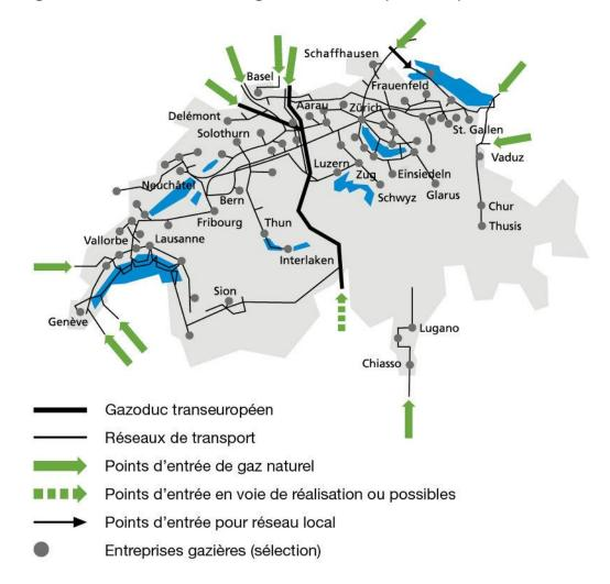
Figure 125 Gas transmission grid Switzerland (overview)
