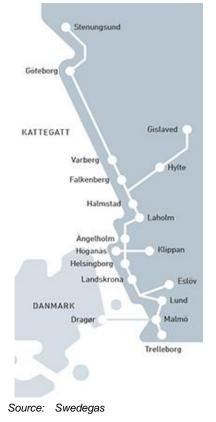
Figure 121 Gas transmission grid in West and South Sweden
