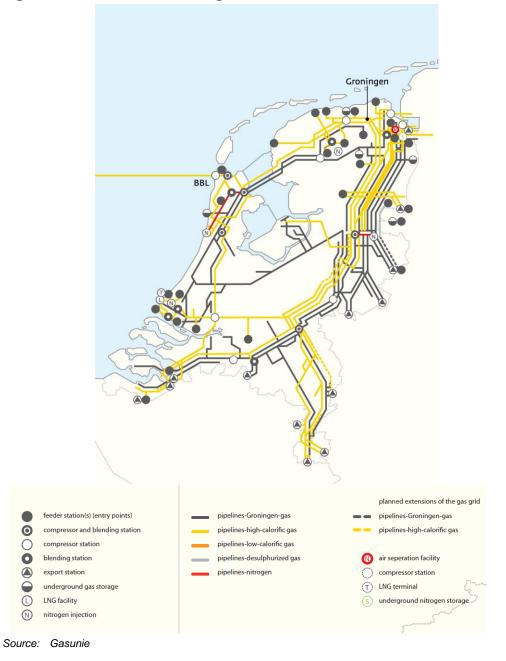
Figure 114 Gas transmission grid in the Netherlands
