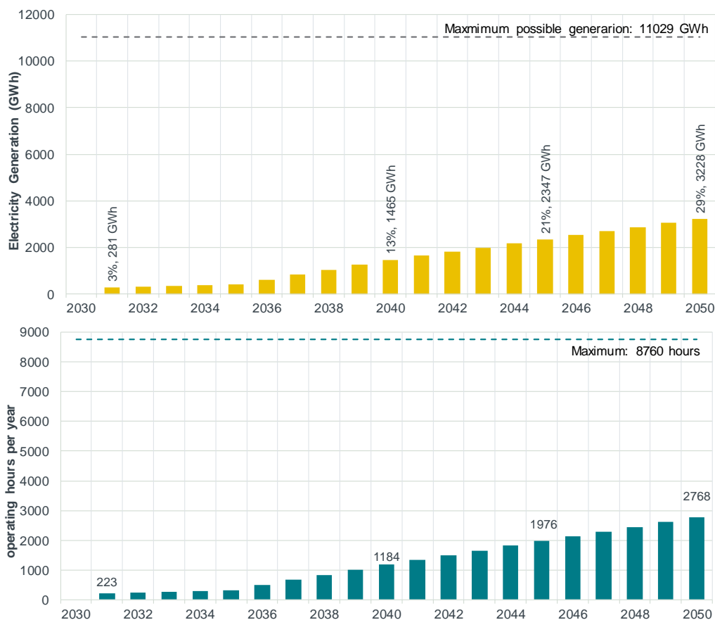
Figure 10 Electricity generation and operating hours of the combined biomass and hydrogen plant
