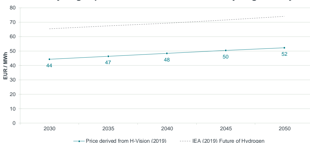
Figure 8 Price of hydrogen derived from H-Vision feasibility study and hydrogen price based on IEA – Future of Hydrogen study
